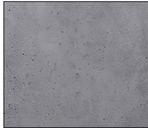
Smooth – Mold Finish No sandblasting straight from the mold
